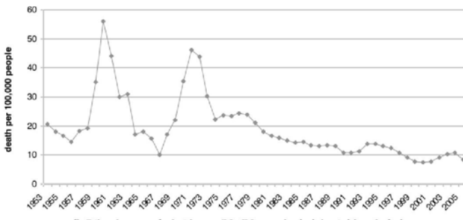
Fig.4 Change of the death number per 100,000 people in industrial and mining enterprises accident, 1953-2005
